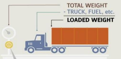
Scales must be certified and calibrated in line with the national standards of the country where the weighing occurred and Method 2 is subject to national certification and approval.
